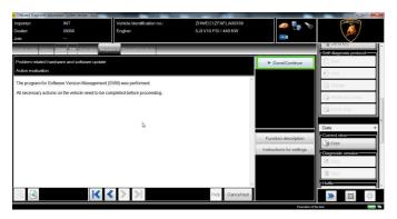
47. Select again the "Special functions" tab and click "Erase fault memory – overall system": this is necessary to delete all errors created during the software update procedure.
